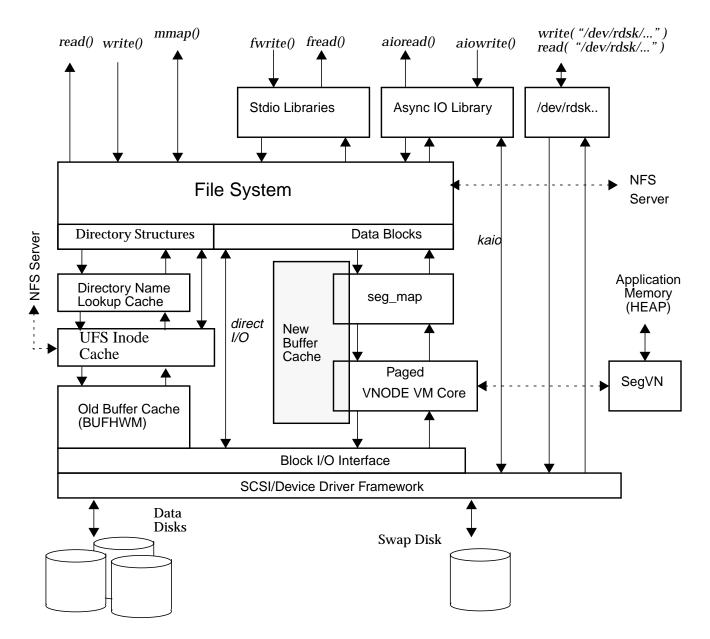
Figure 5-1 Solaris I/O Framework
