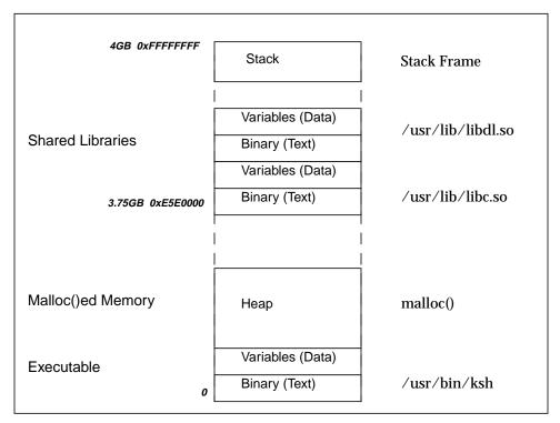
Figure 4-9 Solaris 2.6 Virtual Address Space for a Process
