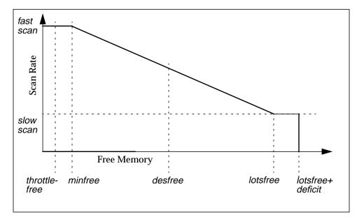
Figure 4-2 Pageout Scanner Parameters
